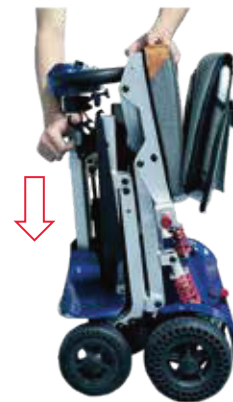
Pull the handle release lever down to release the folding hook.
